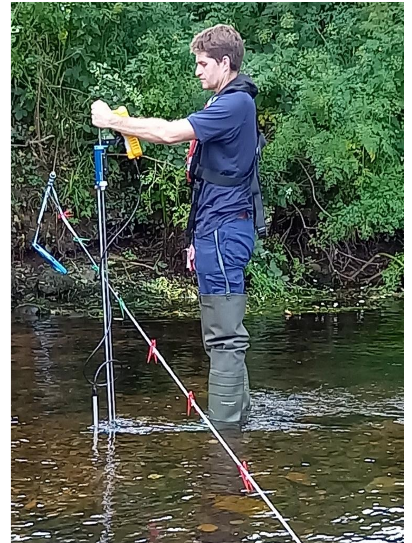
Waded flow measurement with Acoustic Doppler Velocity Meter
